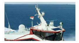
Designed for crew transfers in offshore industries such as wind farms and oil & gas installations, these vessels use powerful fans to generate an air cushion between the catamaran hulls. This unique vessel design, called a "Surface Effect Shp" or SES, minimizes hull drag and resistance to reduce emissions and enhance speed and efficiency. Now, these innovative vessels come with the added intelligence of Sea.Al's Sentry system for enhanced situational awareness at sea.
